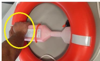
**Step 7:** Firmly press the top side of the plastic body (code 72190) in order to fit in the lifebuoy ring.
