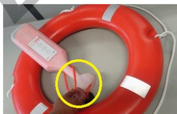
**Step 5:** Pass the plastic body (code 72190) through the rope loop as in the photo.
