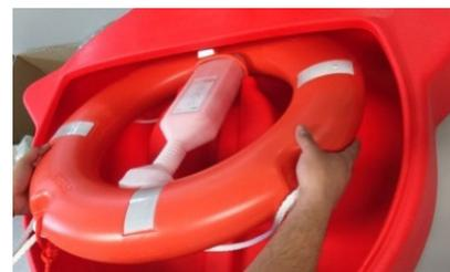
**Step 9:** Place the lifebuoy in the Ring Container.
