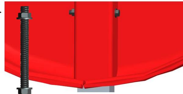
Proposed areas for drilling hole & assemble the M8 bolt & nut is indicated to above photos.
