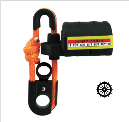
LALIZAS HRU mechanism is designed and produced in the EU (in Greece), in accordance with SOLAS/MED/USCG regulations. It can be easily installed on board, attached to the liferaft according to instructions. The mechanism is automatically activated, in the event of sinking, in a depth of between 1.5 and 4m, allowing the liferaft to be inflated and detached from the sinking vessel. It can be installed to all liferafts of 4-150 persons.
