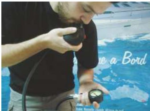
Figure 9 "ON DEMAND" valve operability check
