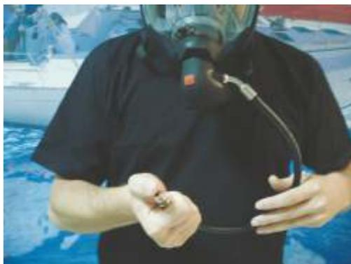
Figure 13 Face piece leak tightness test
