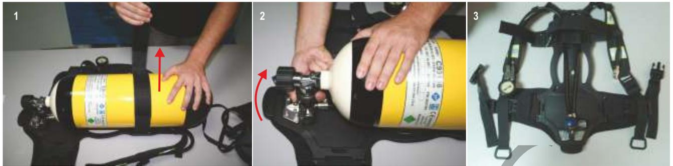
Figure 24 Removal of empty cylinder from apparatus
