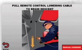
The HLI provides sufficient **guidance** and **real time interaction** between the helmsman and the interface to properly operate lifeboat systems through launch and recovery. It displays **all the necessary texts and animated sequences** to assist the helmsman during those critical moments.
