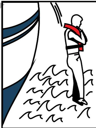
After donning, locate the **Manual lever** for the mechanism; it should protrude from the lifejacket! Make sure that you are comfortable locating it with either hand.
