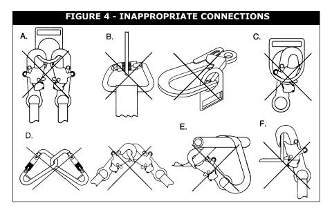
DBI/SALA connectors (snap hooks and carabiners) are designed to be used only as specified in each product's user's instructions. See Figure 4 for inappropriate connections. DBI/SALA snap hooks and carabiners should not be connected:
