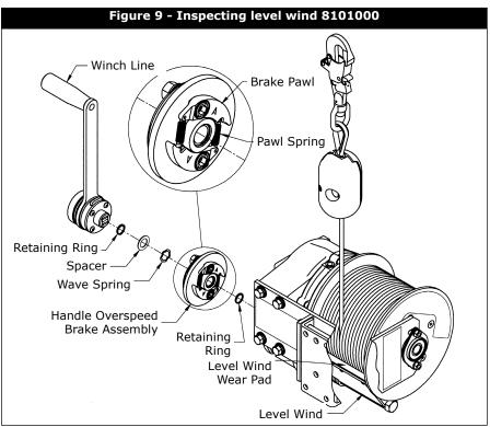
**Step 5.** Check operation of the drum over speed brake as follows, see Figure 9:
