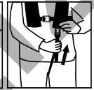
To prevent the lifejacket from riding up on the wearer when in the water, it is vital that the straps are properly adjusted. This may prevent the wearer from being able to maintain their nose or mouth face up above the water surface.
