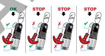
Automatic JS1 inflators can also operate manually, by using their lever.
